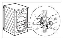
5. Open the door. Remove the polystyrene piece from the door seal and all the items from the drum.
